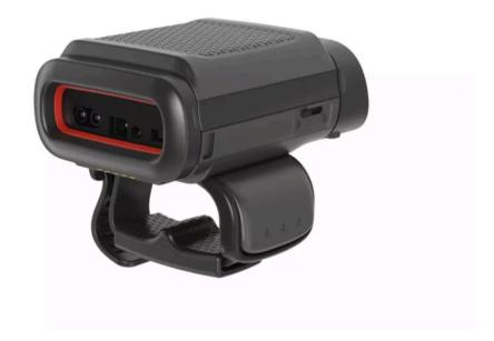
The Honeywell 8680i Wearable Mini Mobile Computer is an advanced compact, ergonomic, high-performance Bluetooth®-wearable scanning solution worn on one hand and designed to help businesses streamline high-volume workflows such as picking, sorting, putaway, and packing for increased speed and efficiency with every transaction.
